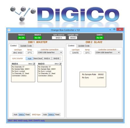
An Orange Box containing two DMI MADI cards can be used to convert 96 kHz MADI between the SMUX and High Speed Formats.
